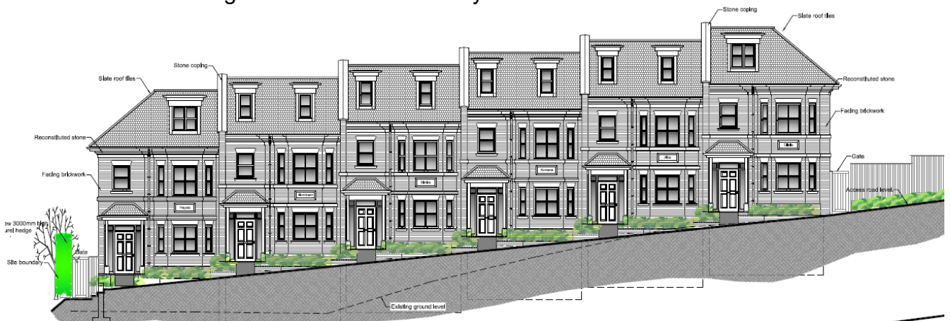
Figure 5. Front elevation plan showing existing levels and proposed level of access road
